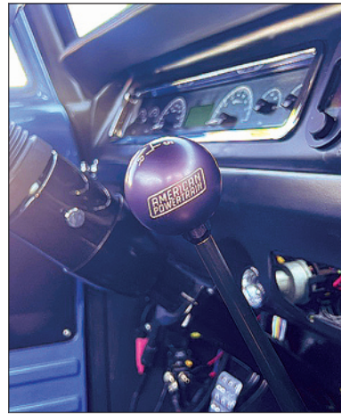
Automatic converted to 5-speed TREMEC (American PowerTrain)
