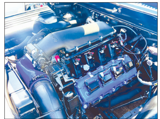
Under the hood: 5.7 Hemi (MDS & VVT deleted) BTR Hemi VVT Stage 4 Camshaft 224x24x, .587/.586, 112.5 LSA Intake Lobe Lift @ TDC: 0.05137
