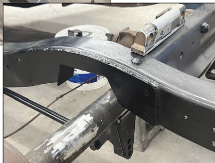
2 & 3. Leaf springs removed. All suspension removed inside the frame. Installed triangulated rear end. Ron and John at Drifters Garage welded in a mini C-notch.
