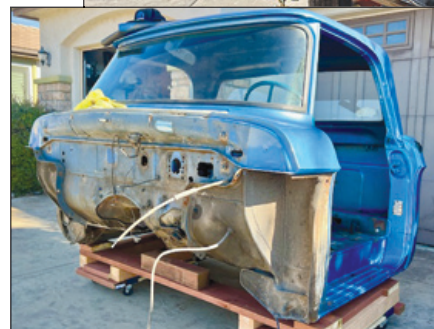
6b. Used my hand grinder and wire wheel to remove all firewall dirt and paint.
