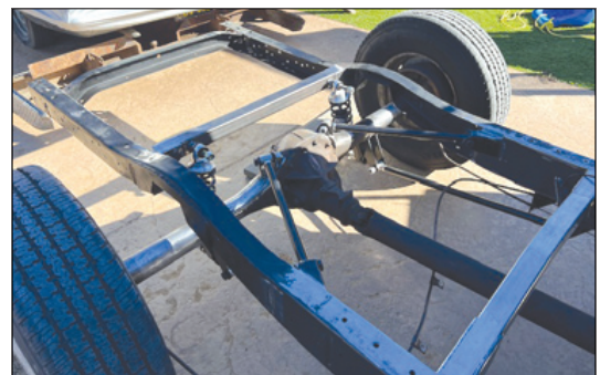
4. Coil over springs added. Look at that wheel and tire space!
