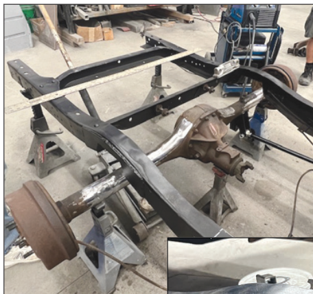
2 & 3. Leaf springs removed. All suspension removed inside the frame. Installed triangulated rear end. Ron and John at Drifters Garage welded in a mini C-notch.
