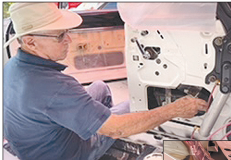
Brad Heavey applying lithium grease to the window regulators
