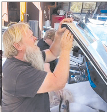
Tim Whittier installing interior window trim
