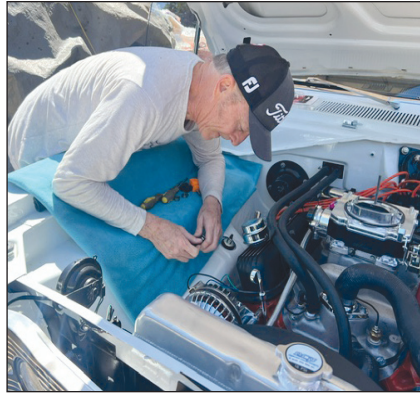
Don Bone installing the fuel filter
