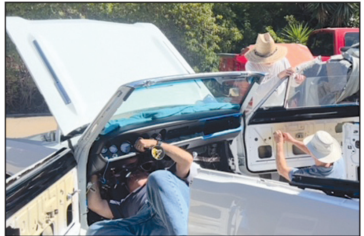
Above, Brad and Don finish re-assembling a window, and below, install it while Jeff tests electrical connections beneath and under the dash
