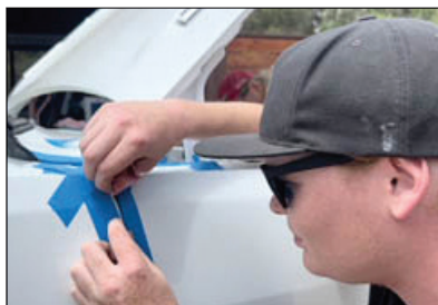
Above, Cam is masking for paint touch-ups. Left, Jim Bowen is wire-wheeling window brackets.
