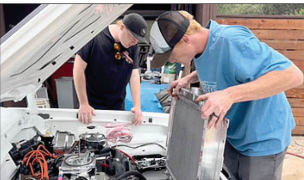
Cam and Cory Whittier remove the radiator in order to attach the chrome overflow reservoir.
