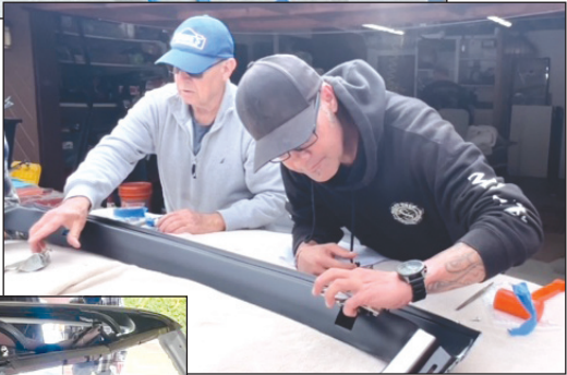
Above, Brad and Peter work through filament interferences between original and new parts for the convertible top. Left, the completed convertible top skeleton.
