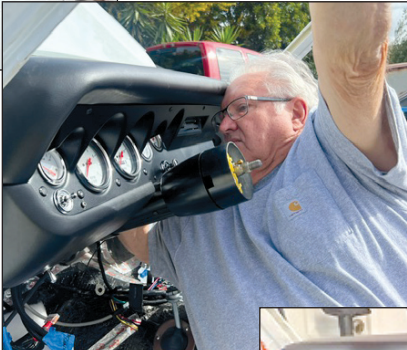
Above, Jeff wrestles with connecting the oil pressure line to the oil pressure gauge behind the dash.
