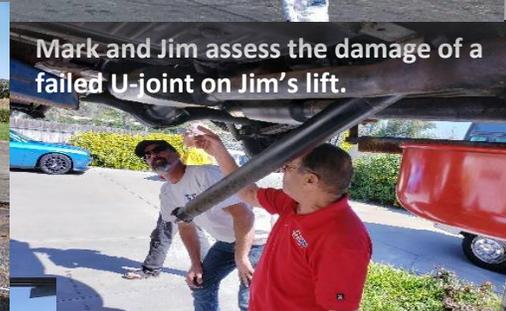
Mark and Jim assess the damage of a failed U-joint on Jim's lift.
